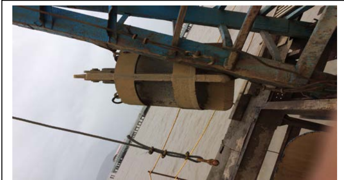
Fig. 17. Sharp edge chisel 3.5ton capacity
