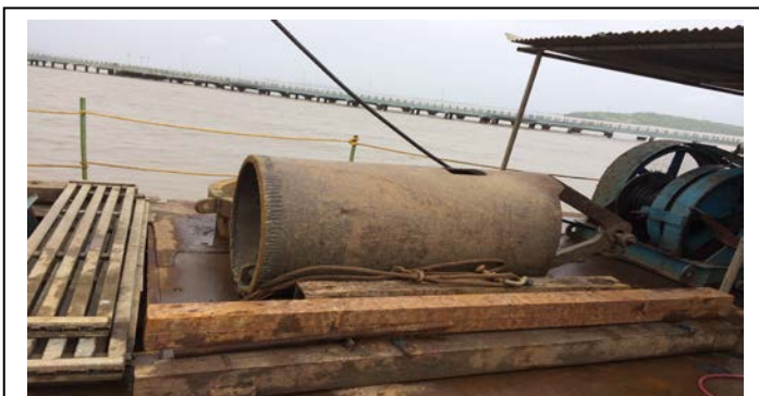
Fig. 19. Bailer, one way opening 0.5m3 capacity
